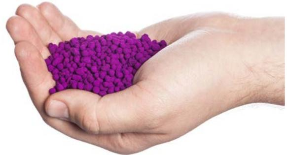
**Purafil SP Media** consists of generally spherical, porous pellets formed from a combination of activated alumina and other binders, suitably impregnated with sodium permanganate ( $\text{NaMnO}_4$ ). The sodium permanganate is applied during pellet formation such that it is uniformly distributed throughout the pellet volume and is completely available for reaction with target gases.
